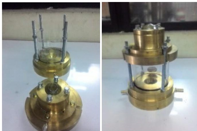
Figure 7. The process of assembling an electric arc furnace
