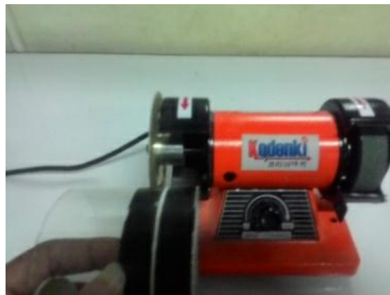
Figure 5. Glass cutting machines speed 0-9900 rpm
