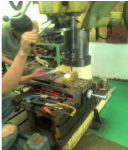
Figure 3. Drilling of cooling holes
