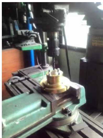
Figure 6. Drilling ball drive TIG welding gun
