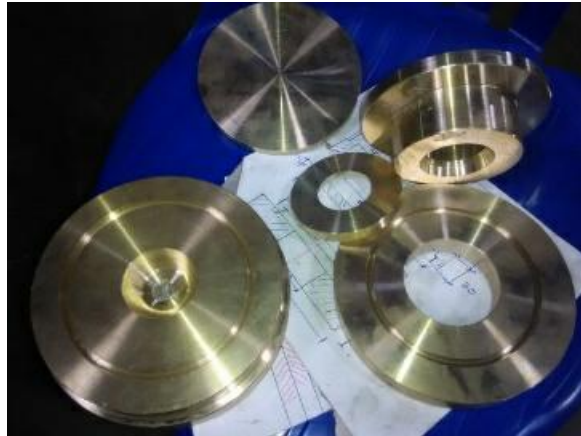
Figure 2. Molded brass furnace after machining
