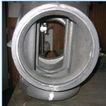
Figure 13: Grey cast iron casting, the core is made from GEOPOL® CO 2 sand mixture.
