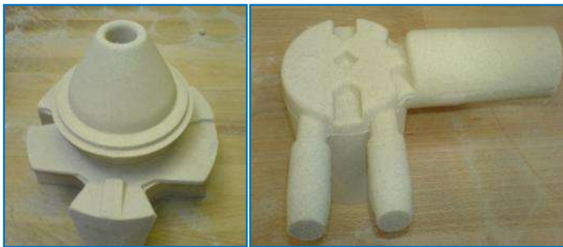
Figure 12: Small cores made on the core shooting machine, addition level: 100 weight parts of sand ST55, 3.0 weight parts of GEOPOL® binder, 0.7 weight parts of GEOTEK accelerator.
