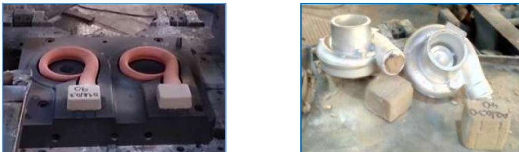
Figure 16: Coated cores cored to the metal mould (left). Castings after pouring (right).
