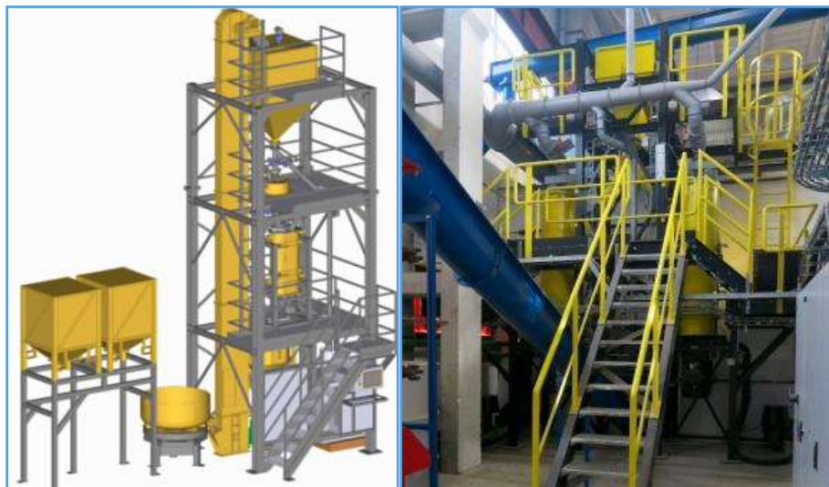
Figure 21: Reclamation plant assembly scheme with primary and secondary reclamation (left), only secondary reclamation stage (right).
