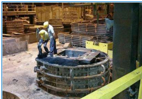
Figure 8: Production of the large moulds using polystyrene patterns.
