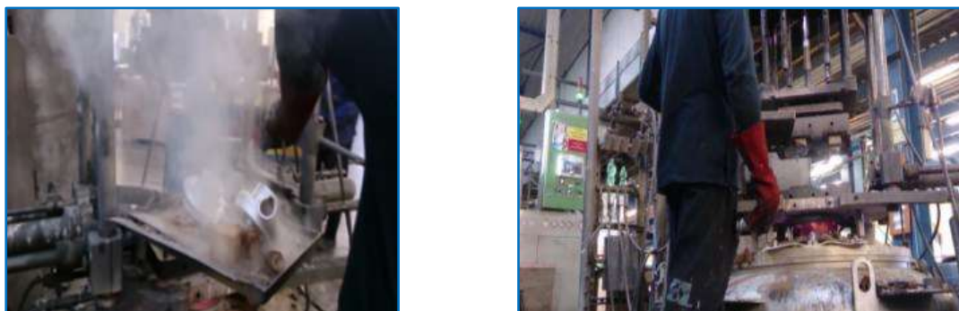
Figure 17: Comparison of gas evolution after pouring. Castings immediately after pouring, the PUR cold box amine technology (organic binder)(left). Opening of the die immediately after pouring, cores made by GEOPOL® W technology (inorganic binder)(right).
