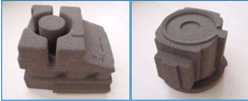
Figure 5: Smaller cores made from 100% reclaimed sand by the GEOPOL ® technology, the self-hardening sand mixture.
