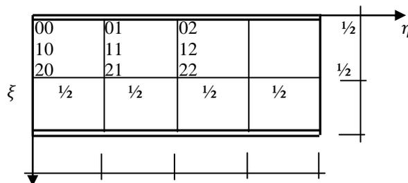
**Figure 3: rectangular plate ( $b = 2a$ ) with two parallel articulated edges and two parallel free edges**
