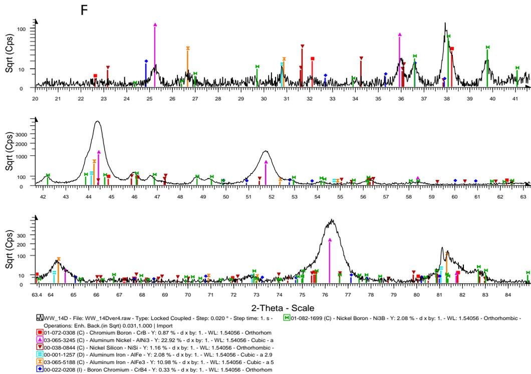
Figure 8 XRD patterns of the fracture surface of the Fe<sub>3</sub>Al/BNi-2/steel joint Bonded at: T<sub>b</sub> = 1040 °C and t<sub>b</sub>= 5 minutes.
