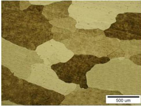
Figure 1 Optical micrograph of Fe<sub>3</sub>Al (100x).
