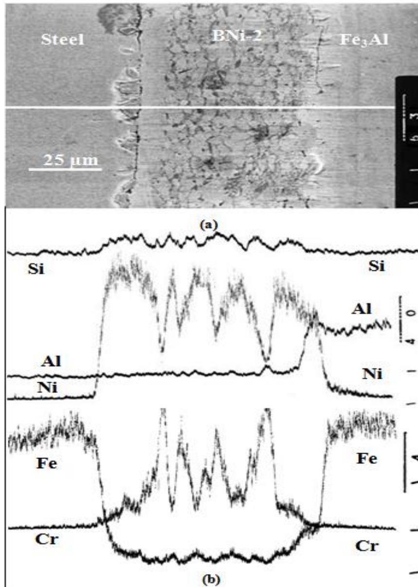
Figure 6 EPMA line analysis across the  $Fe_3Al/B-Ni83/steel$  joint bonded at:  $T_b=1040\text{ }^\circ\text{C}$  and  $t_b=5\text{ min}$ :
