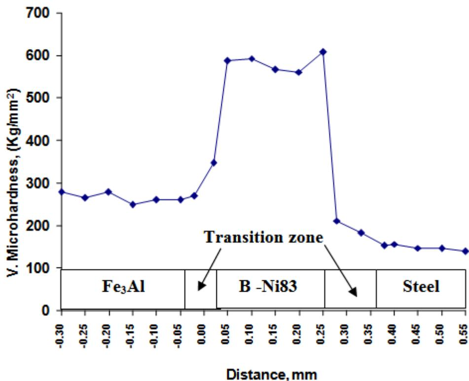
Figure 4 Vickers Microhardness of Fe<sub>3</sub>Al/BNi-2/steel joint bonded at:  $T_b=1040$  °C;  $t_b= 5$
