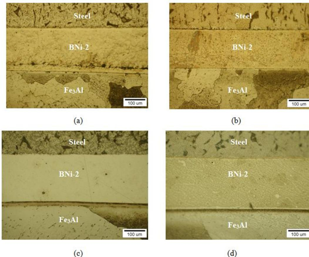
**Figure 5** Optical micrograph of cross-section of  $Fe_3Al$ /BNi-2/steel joint bonded at:  $T=1040\text{ }^{\circ}\text{C}$  and at: (a)  $t_b=2\text{ min}$ . (b)  $t_b=5\text{ min}$ . (c)  $t_b=10\text{ min}$ .  $t_b=20\text{ min}$ . x200.
