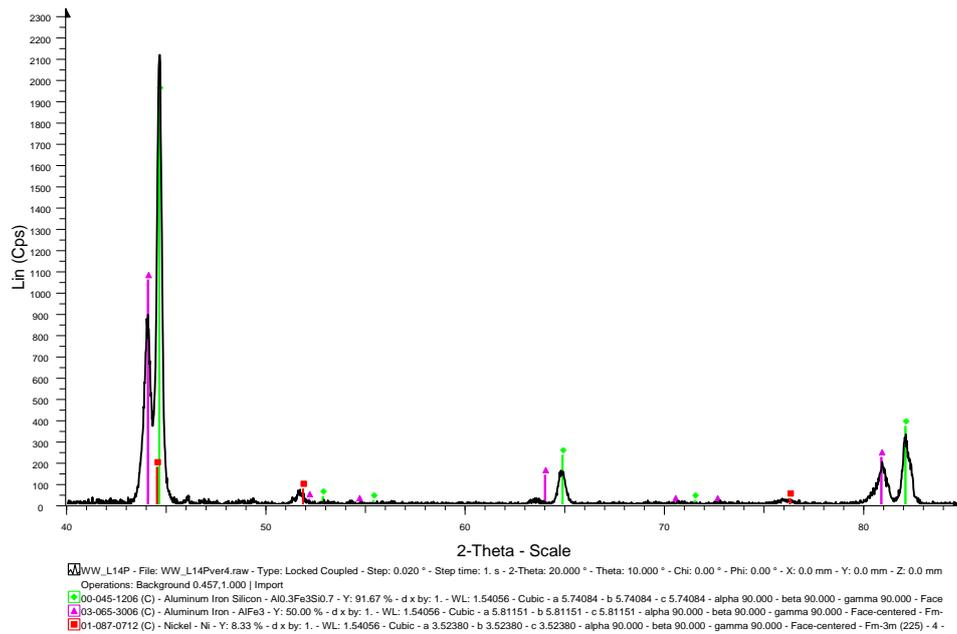
Figure 7 XRD patterns of the cross- section of the Fe<sub>3</sub>Al/BNi-2/steel joint Bonded at: T<sub>b</sub> = 1040 °C and t<sub>b</sub>= 5 minutes.
