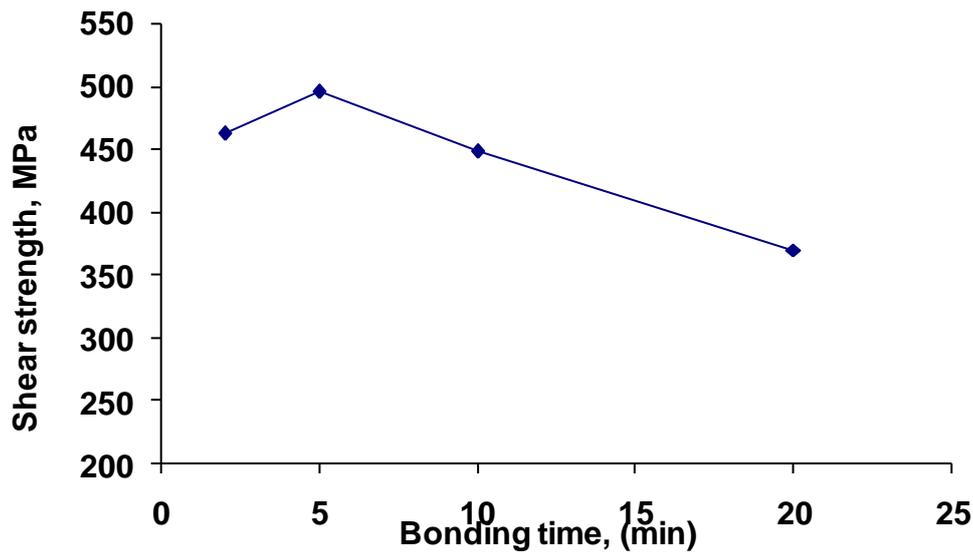
Figure 3 The effect of holding time on the joint strength of Fe<sub>3</sub>Al/BNi-2/steel joints bonded at:  $T_b=1040$  °C.
