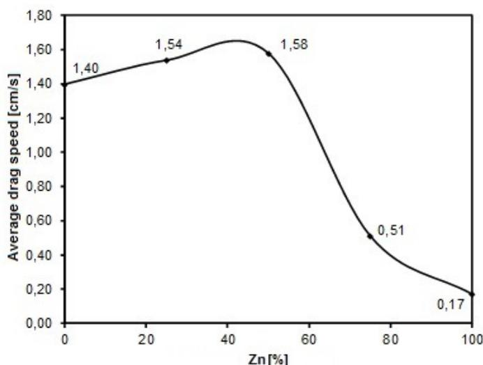
Figure 4– Average drag speed of the samples as a function of Zn concentration.
