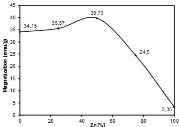
Figure 3– Saturation magnetization of the samples as a function of Zn concentration.
