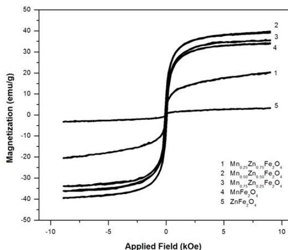
**Figure 2– Magnetization of the samples as a function of the applied field.**
