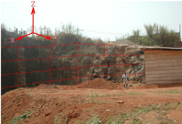
Figure 5 : Grid following the cracks on the outcrop of Cité-verte (N03°52'37,8'' ; E11°28'49,0'' ; H = 813 m) [25]
