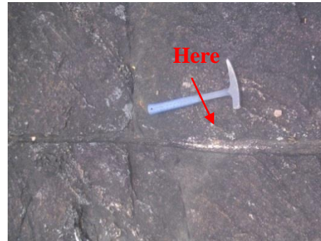
Photo 6 : Quartzo-feldspathic filled joints, materializing an episode of brittle tectonic
