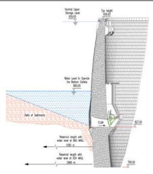
**Principle-** If the water level is reduced, the reservoir is full with sediment laden water. If as such the sluice gate is opened there will be discharge of the sediments.
