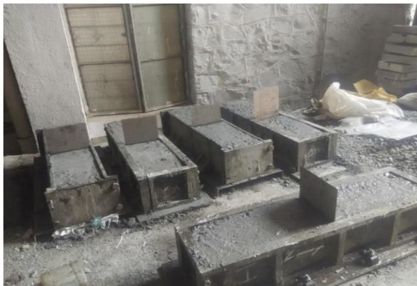
Fig. 3. Casting and development of artificial notch using ply-wood.
