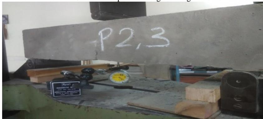
Fig. 2. Experimental set-up for three point bend test.
