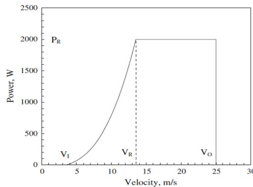
Fig.3 Theoretical Power curve of a 2MW wind turbine
