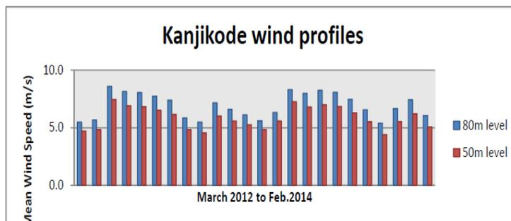
Fig.1 Kanjikode wind profiles at different hub heights
