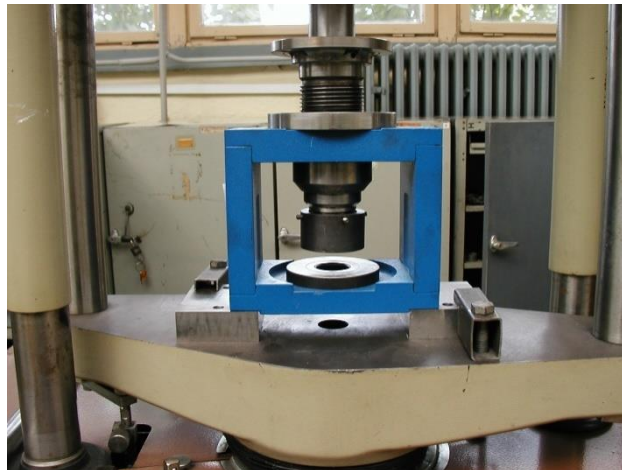
Fig. 3 Cupping test tool
