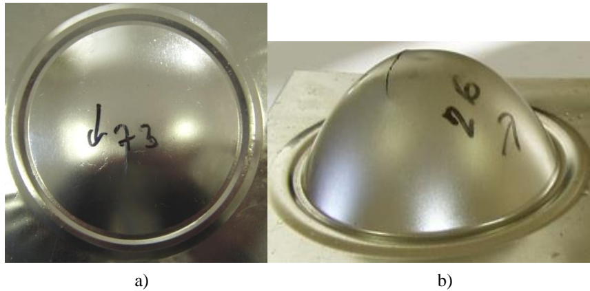
Fig.2 Sample after biaxial tension test of TS 480 BA (a), TS 275 BA (b)
