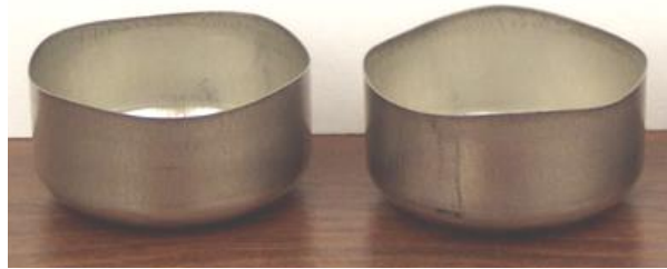
Fig. 4 Samples after cupping test
