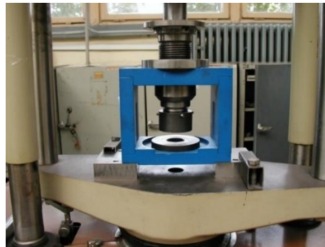
Fig. 1 Deep-drawing tool for cupping test
