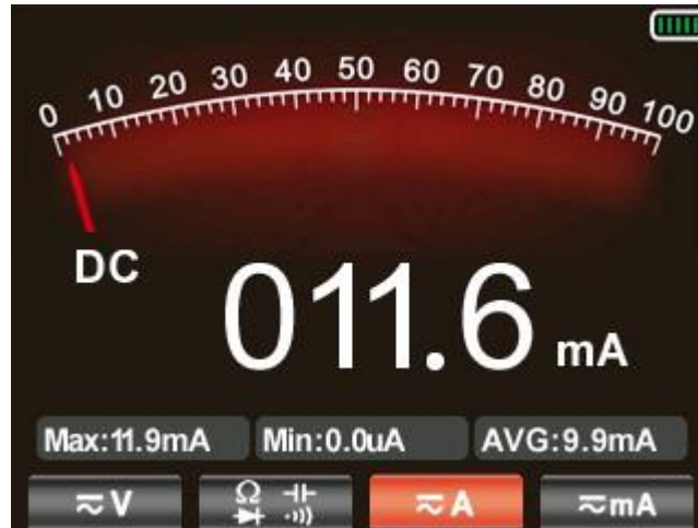
Figure 8 Working current of the GP2Y0A41SKOF
