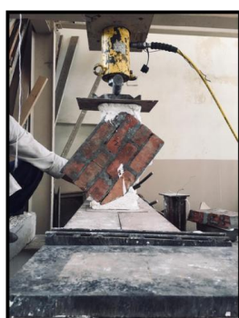
a. Prism constructed using mortar TW.
