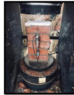
b. Prism constructed using mortar STWW.
