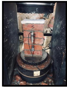
a. Prism constructed using mortar TW.
