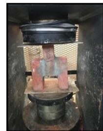
b. Prism constructed using mortar STWW.
