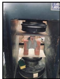
a. Prism constructed using mortar TW.
