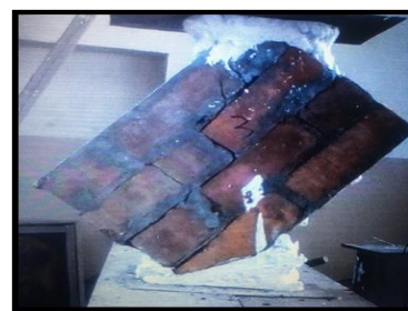
b. Prism constructed using mortar STWW.
