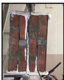
a. Prism constructed using mortar TW.
