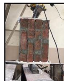
b. Prism constructed using mortar STWW.
