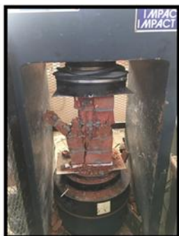
a. Prism constructed using mortar PW.
