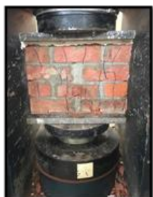
a. Prism constructed using mortar PW.
