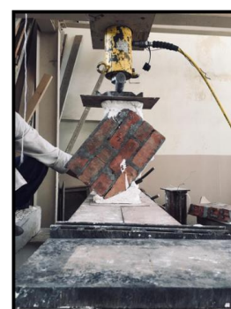
b. Prism constructed using mortar STWW.
