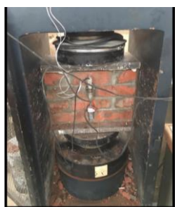
a. Prism constructed using mortar TW.
