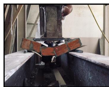
b. Prism constructed using mortar STWW.
