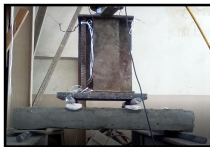
b. Prism constructed using mortar STWW.
