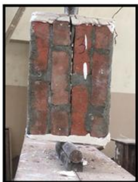
a. Prism constructed using mortar PW.
