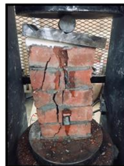
b. Prism constructed using mortar STWW.
