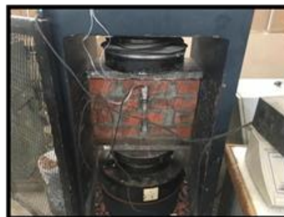
b. Prism constructed using mortar STWW.
