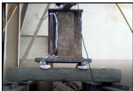
a. Prism constructed using mortar TW.
