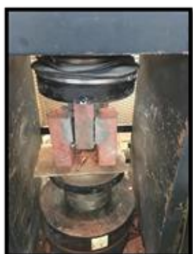
a. Prism constructed using mortar PW.
