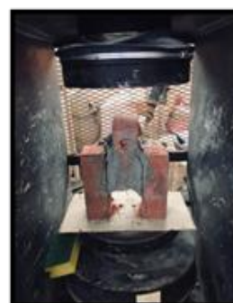
b. Prism constructed using mortar STWW.
