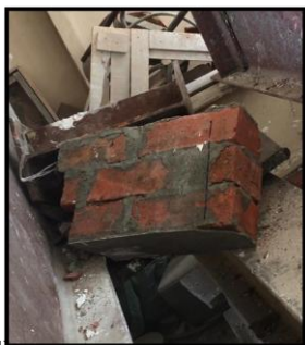
Fig. 17: Failure mode of out of plane bending-tension parallel to bed joints.
