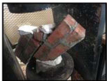
a. Prism constructed using mortar TW.
