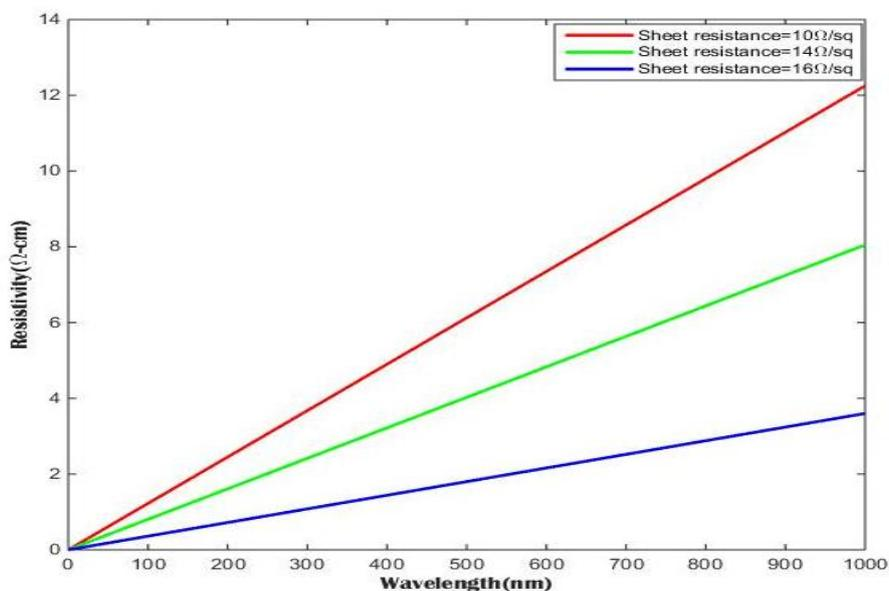
Fig. 4: ITO films simulated resistivity as a function of increasing sheet resistance
