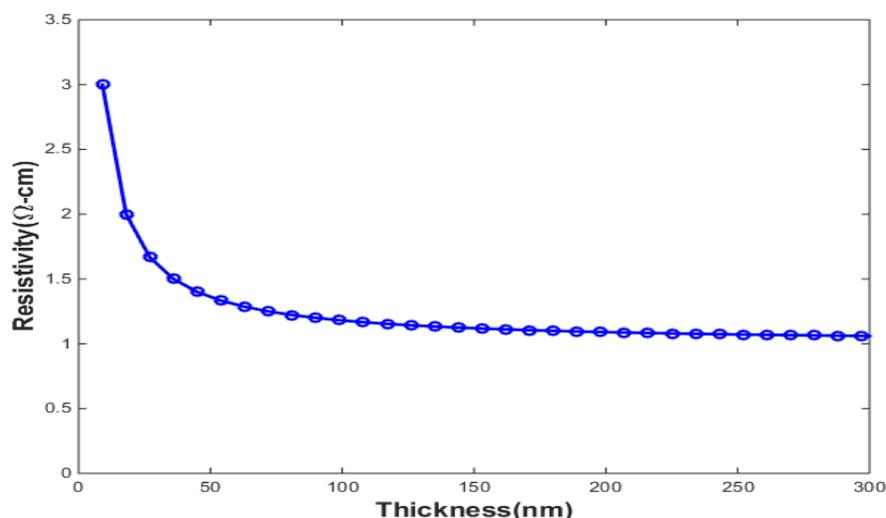
Fig. 5: ITO films resistivity against optical thickness
