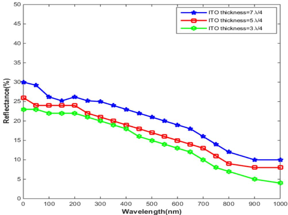
Fig. 2: ITO films optical reflectance with respect to films thickness
