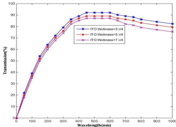
Fig. 1: ITO films optical transmission with respect to wavelength as a function thickness
