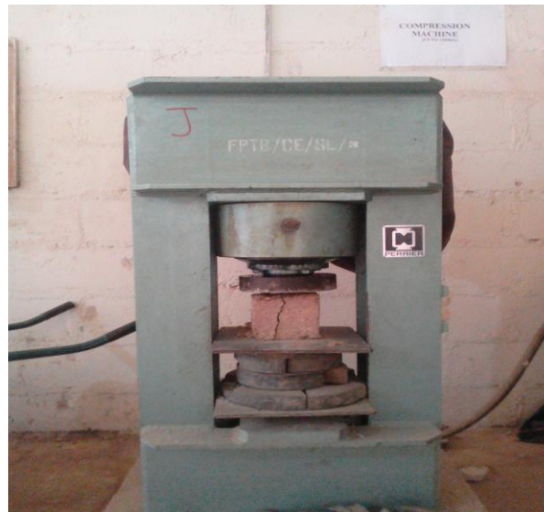
Plate 1: Crushing of cube to determine compressive strength in the laboratory
