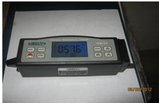
Plate 4: Surface Roughness Tester, ISR-16
