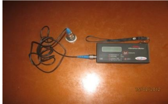
Plate 3: Vibration Meter with Transducer, 908 BE
