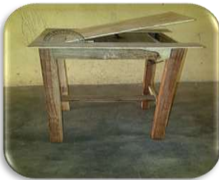
Fig.2: A drafting table to determine coefficient of static friction Fig. 3: An apparatus for measuring angle of repose
