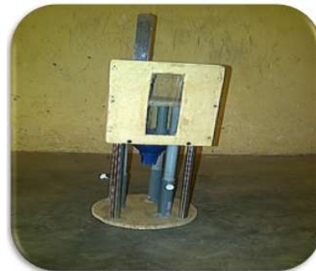
Fig.2: A drafting table to determine coefficient of static friction Fig. 3: An apparatus for measuring angle of repose
