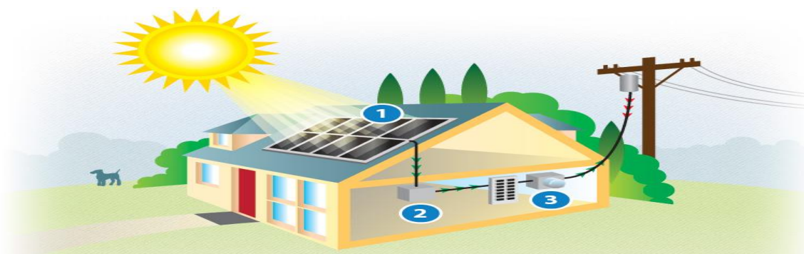
Figure1: Proposed direct grid-connected PV System [14]
