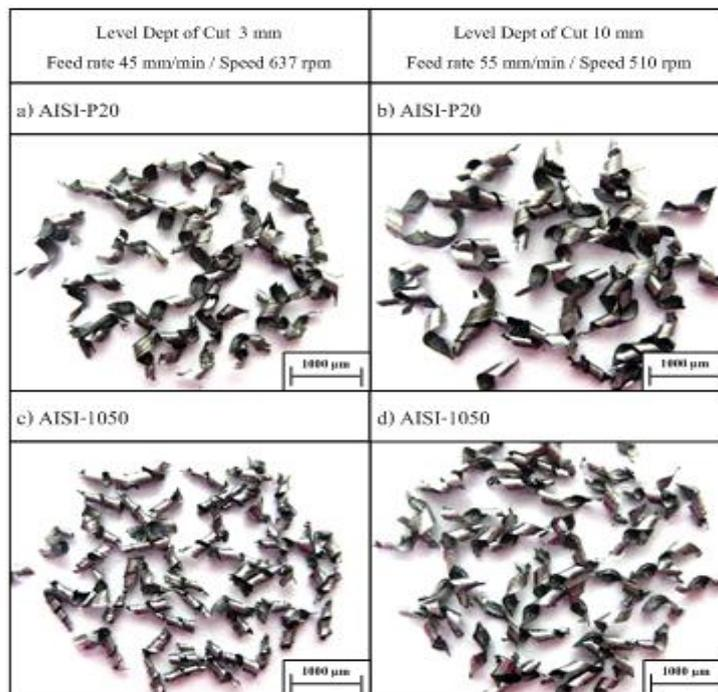
Fig. 8 Characteristic of machined chip of plastic mold steel AISI-P20 and AISI-1050
