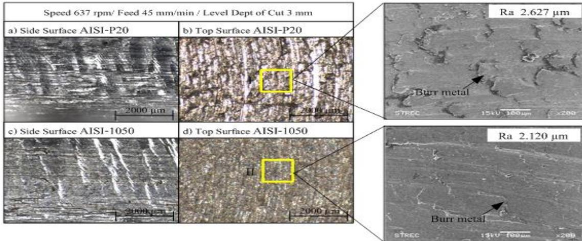
Fig. 3 SEM magnified 200x of the good surface quality for milling surface
