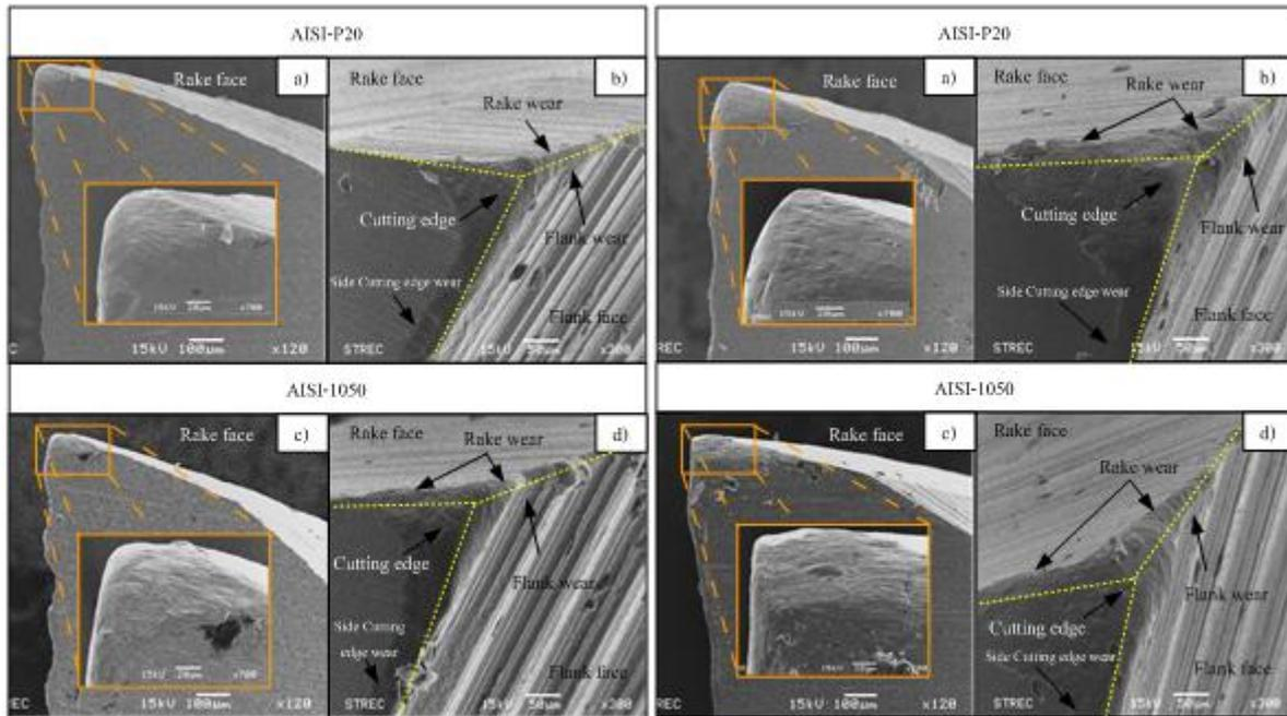
**Fig. 10** Characteristic of less cutting edge wear
