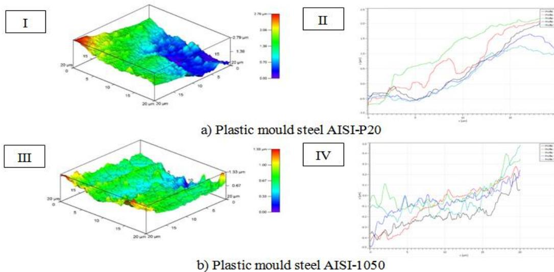
Fig. 7 Characteristic of the poor surface quality measured by AFM
