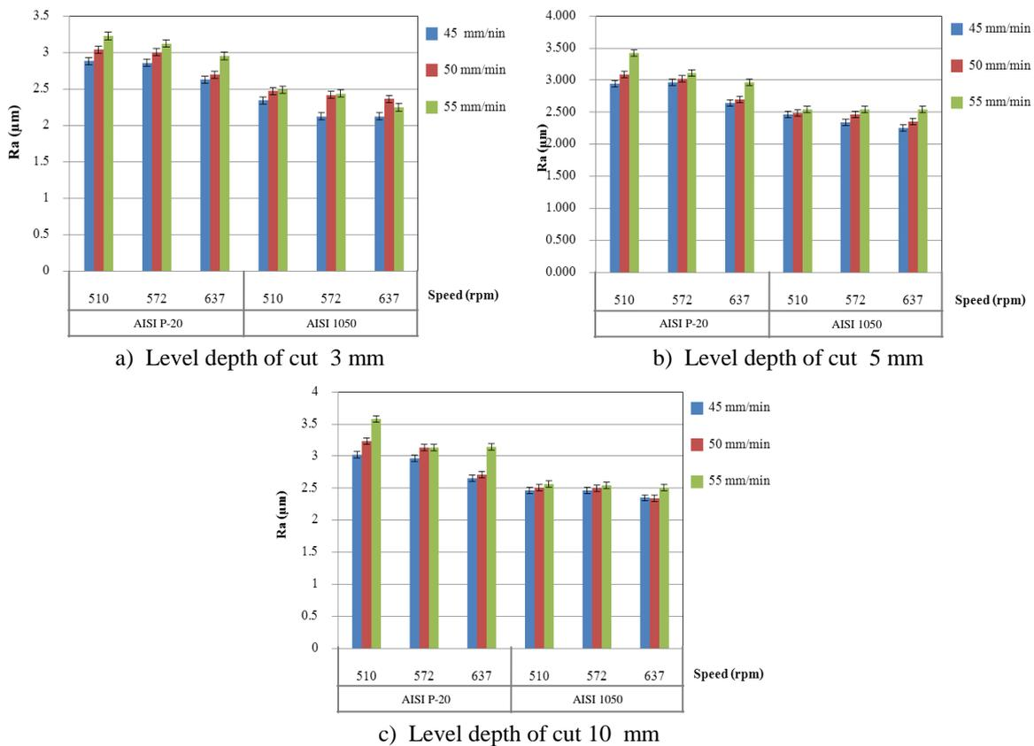
Fig. 2 Arithmetic average roughness (Ra) provided
