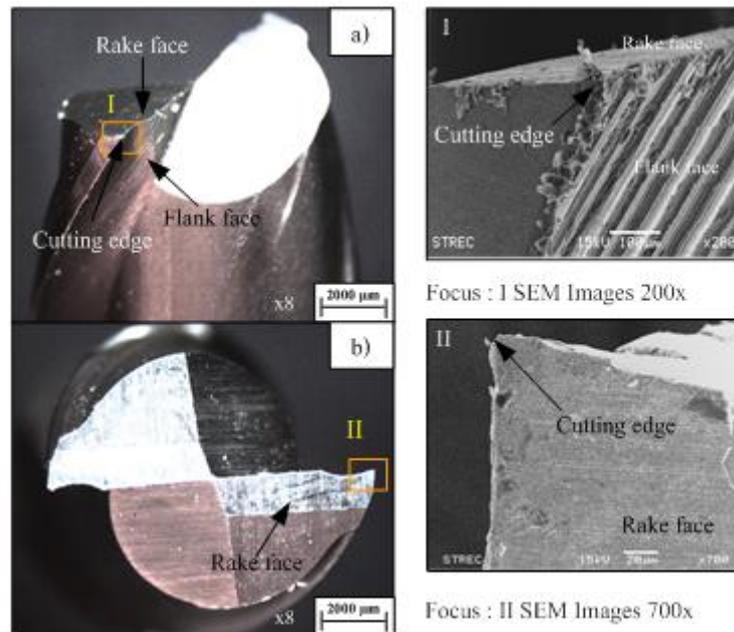
**Fig. 9** Measured positions on cutting edge wear
