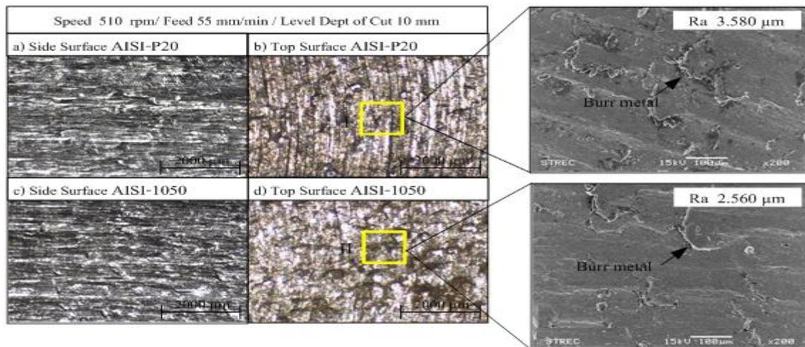
Fig. 4 SEM magnified 200x of the poor surface quality for milling surface
