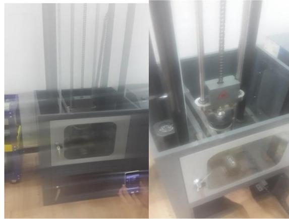
Figure (7) Impact test system of drop weight.
