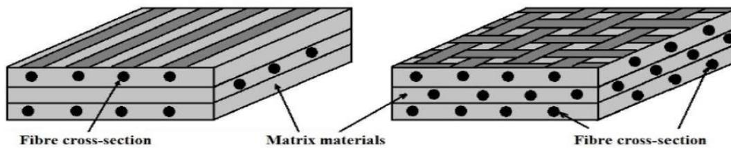
Figure (1) illustration the formation composite materials by using fiber and matrix [1].
