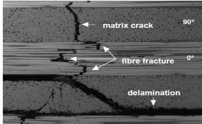
Figure (4) Cross-section view of the impact damaged composite laminates <sup>[12]</sup>.
