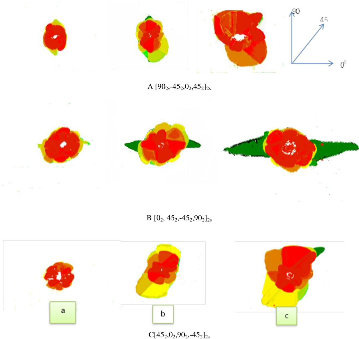
Figure (10) delamination area (a) impact energy 15J (b) impact energy 25 J (c) impact energy 35 J
