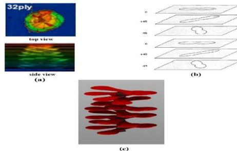
Figure (5): (a) Top and side views of the delamination area from C-scan observations <sup>[12]</sup>; (b) schematic illustration of delamination <sup>[8]</sup>; (c) ideal model of delamination <sup>[12]</sup>.
