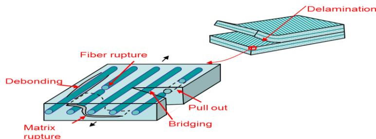
Figure (6) the mechanism of failure modes of composite materials under low velocity impact <sup>[13]</sup>.
