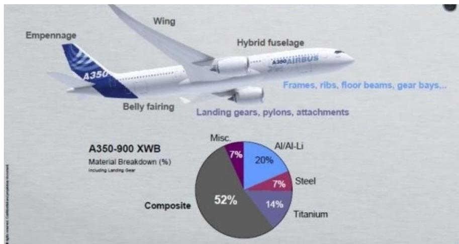
Figure (2) Airbus A350 Distribution of material [6].
