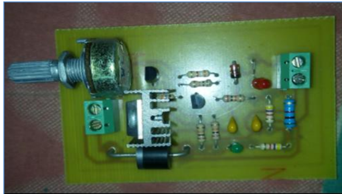
Figure 6: Charge Controller Prototype.
