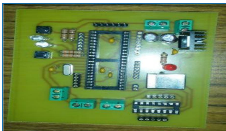
Figure 7: PIC Bootloader circuit for this project.
