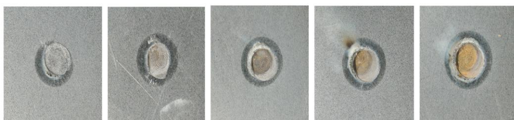
Figure 4: Welding electrodes indentations of Samples A (H220PD + H220PD): a) I=4 kA, b) I=5 kA, c) I=6 kA, d) I=7 kA, e) I=8 kA
