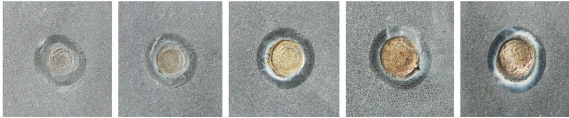
Figure 5: Welding electrodes indentations of Samples B (H220PD + TRIP40/70): a) I=5kA, b) I=6kA, c) I=7kA, d) I= 8kA, e) I=9kA
