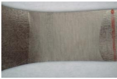
Figure 5: Inhomogeneity of plastic deformation
