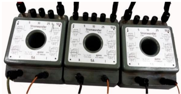
Figure 4: The current transformers (CT's)
