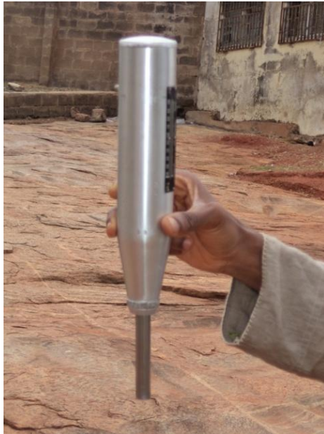
Plate 1: The rebound hammer used for the study.
