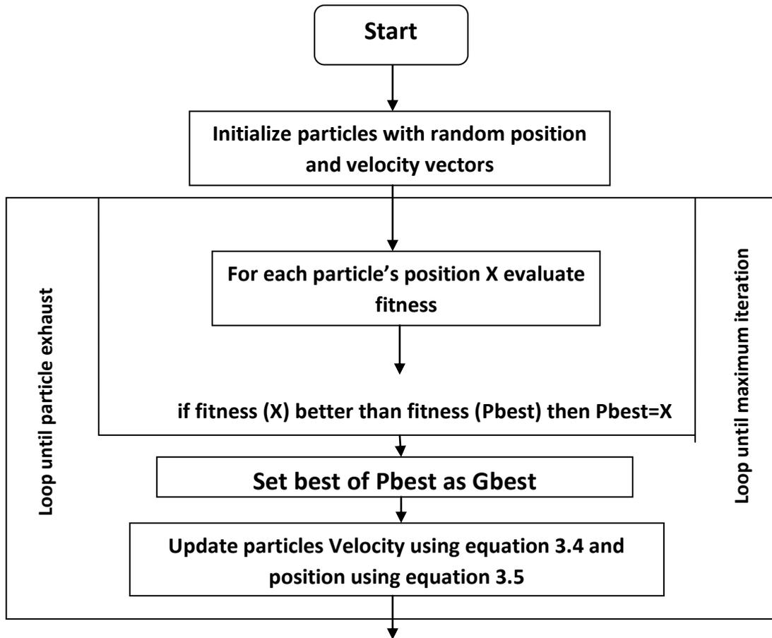
$$V_i^{k+i} = V_i^k + c_1 r_1 (Pbest_i^k - X_i^k) + c_2 r_2 (Gbest_i^k - X_i^k) \quad 3.4$$
