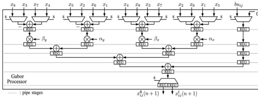
Fig.2. Logical block diagram of one CNN-based GTF computation unit
