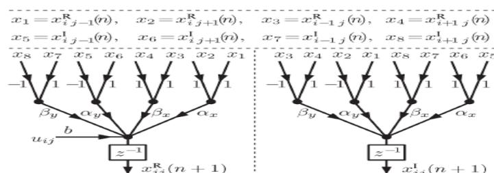
Fig.1 DT-CNN-based GTF structure signal flow graph [22]
