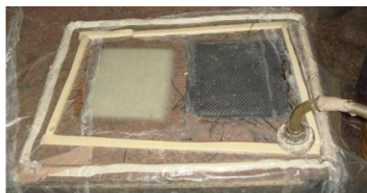
Fig: 1 Vacuum Bagging Technique
