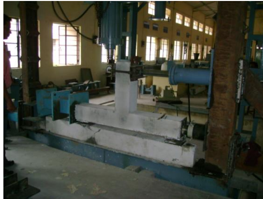
Fig.3 Test setup showing Beam column joint with required arrangements
