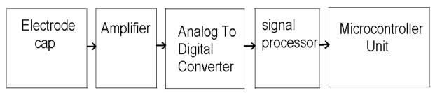
Fig2 : General Block Diagram of the Proposed System
