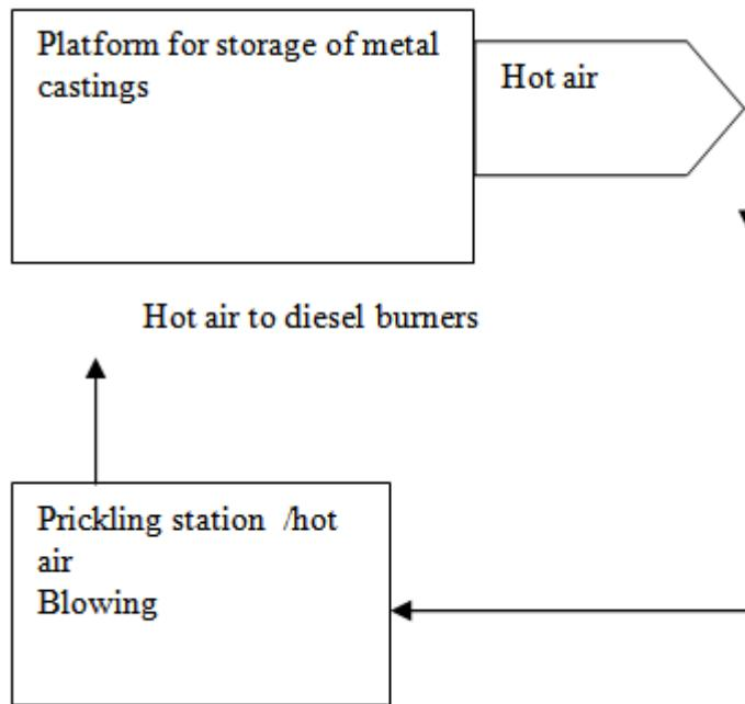
The annual saving in above arrangement is estimated to be 45 KW of electricity with total 224640 units of electricity at the @ 16 hrs per day effective operation of heaters and factory operating 6 days a week. The total cost saving will Rs 1347840.00 with investment of Rs800000. The total saving due to above is 1347840.00 and pay back period is 0.59 years.
