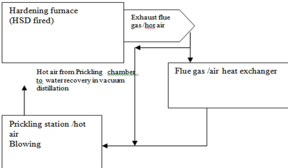
(ii) Alternatively the hot quenching water of die casting in melting furnaces available at 50°C can be circulated through a water to air heat exchanger to preheat the air before further passing it over the rolled coils to gain further temperature before finally passing it through prickling station .The blown air in hot drying chamber can be led to the Air pre heater of furnaces and then to burners or for water recovery as suggested in at (i) above..
