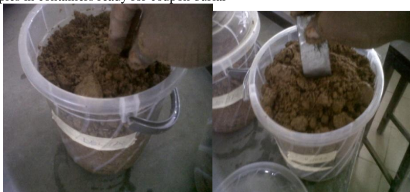
Fig. 2: Burial of coupon in soil samples
