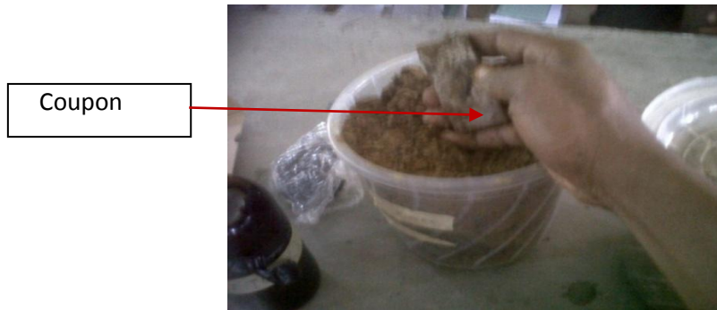
Fig. 3: Retrieval of one of the coupons from soil
