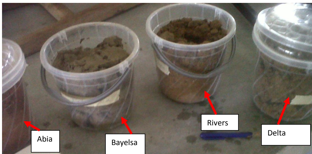
Fig. 1: Soil samples in containers ready for coupon burial
