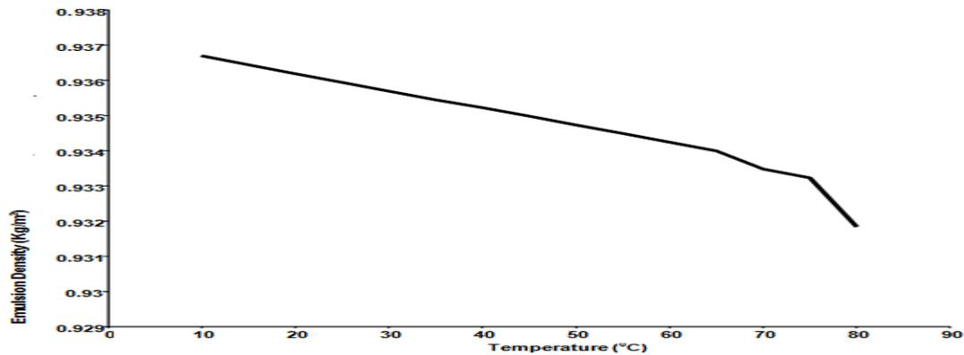
**Figure 7 Density of fluted pumpkin seed oil emulsion extracted with n-hexane at 1 bar atmospheric pressure as a function of temperature.**
