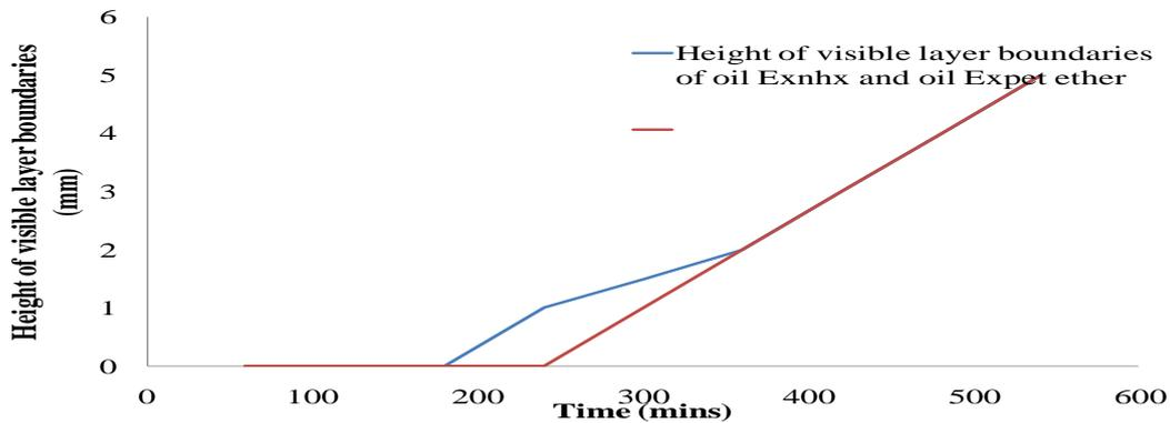
Figure 4 Time dependent height increase of the visible creaming layers of olive oil, oil extracted with n-hexane and petroleum ether.
