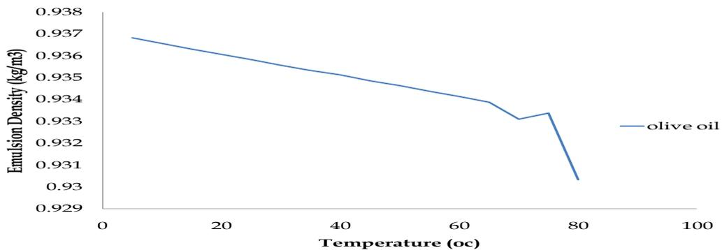
Figure 5 Density of Olive Oil emulsion at 1 bar atmospheric pressure as a function of temperature.
