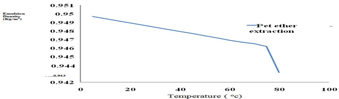
Figure 6 Density of fluted pumpkin seed oil emulsion extracted with petroleum ether at 1 bar atmospheric pressure as a function of temperature.
