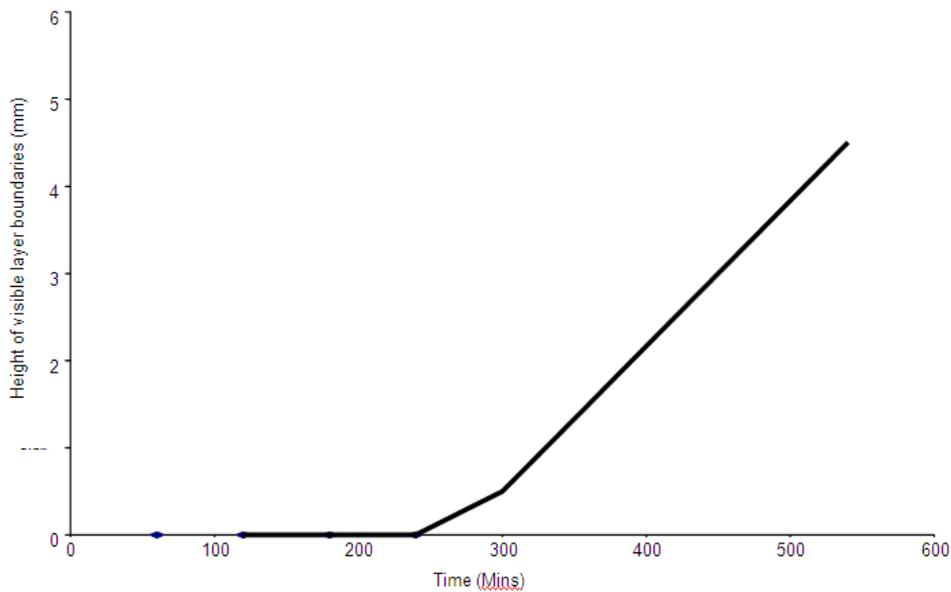
**Figure 3 Time dependent height increase of the visible creaming layer boundary of oil extracted with n-hexane.**
