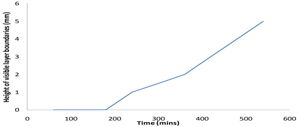
**Figure 2 Time dependent height increase of the visible creaming layer boundary of oil extracted with petroleum ether.**
