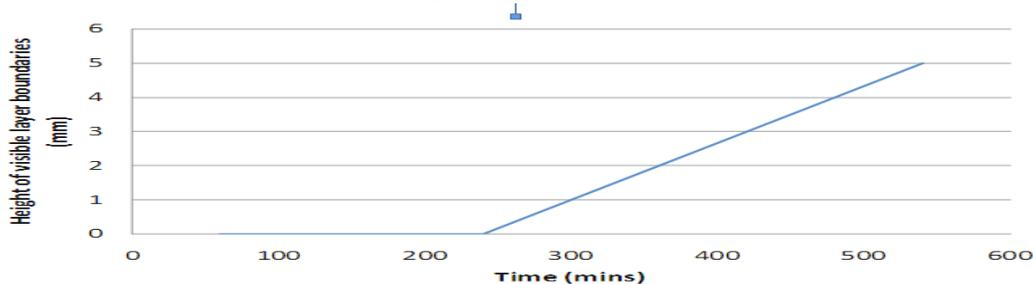
**Figure 1 Time dependent height increase of the visible creaming layer boundary of olive oil emulsion.**
