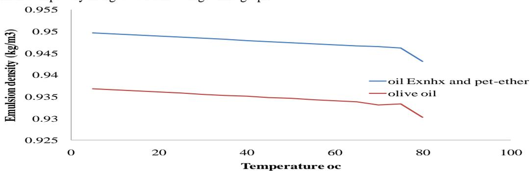
**Figure 8 Density of olive oil, oil extracted with n-hexane and petroleum ether emulsions at 1 bar atmospheric pressure as a function of temperature.**
