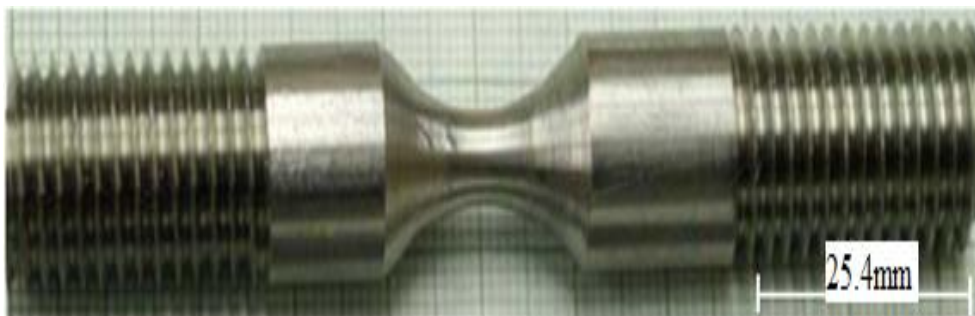
Figure 1. Fatigue test specimen before testing.
