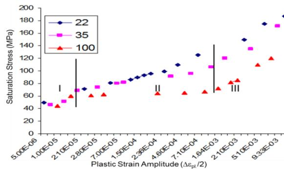
Figure 2: CSS Curves of Copper with grain sizes of 22 $\mu\text{m}$ , 35 $\mu\text{m}$ , and 100 $\mu\text{m}$ .
