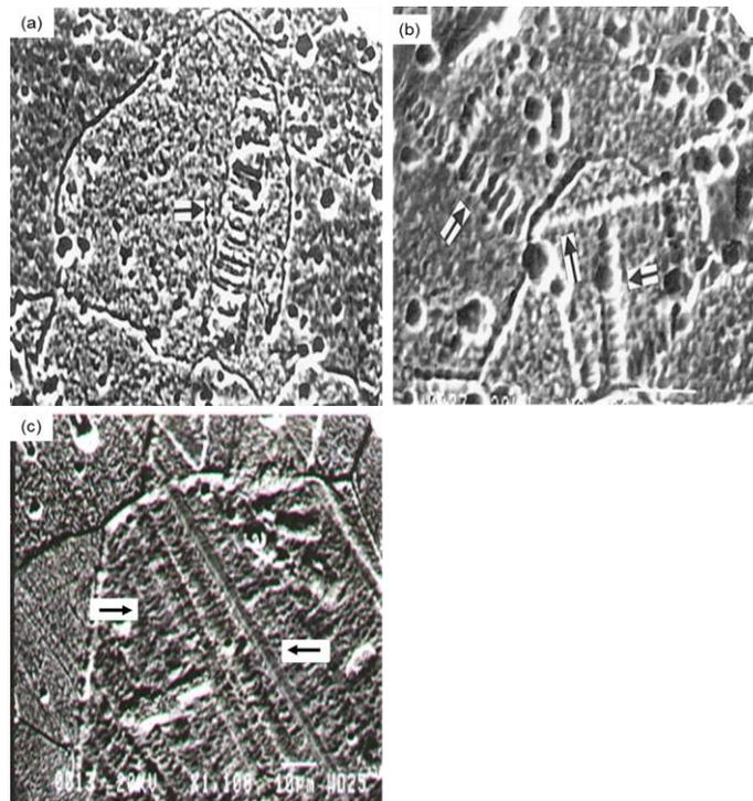
Figure 3: SEM micrographs showing (a) less PSB's for 22 $\mu\text{m}$  grain size, (b) more PSB's for 35 $\mu\text{m}$  grain size, and (c) fully filled with PSBs for 100 $\mu\text{m}$  grain size. All samples were taken from the intermediate region (II).
