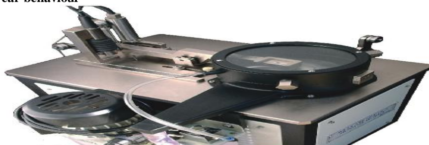
Fig.4. Set up of pin-on-disc wear testing machine
