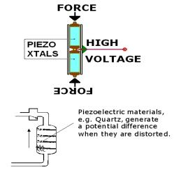
Piezoelectric generation of charge
