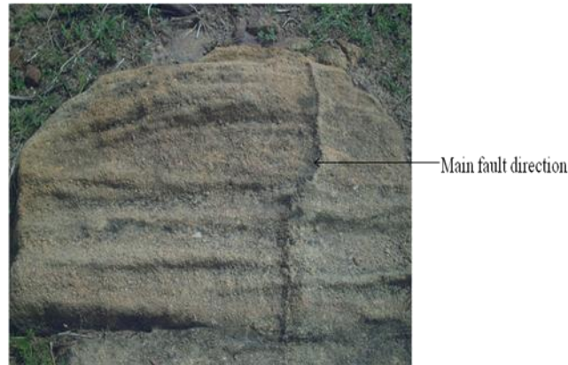
Plate 1: Deformation bands associated with fault on Bima Sandstone (notice the fault perpendicular to the bands)
