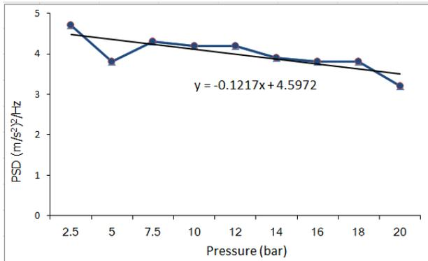
Fig. 4(b) Effect of applied load on vibration at 17km/hr.
