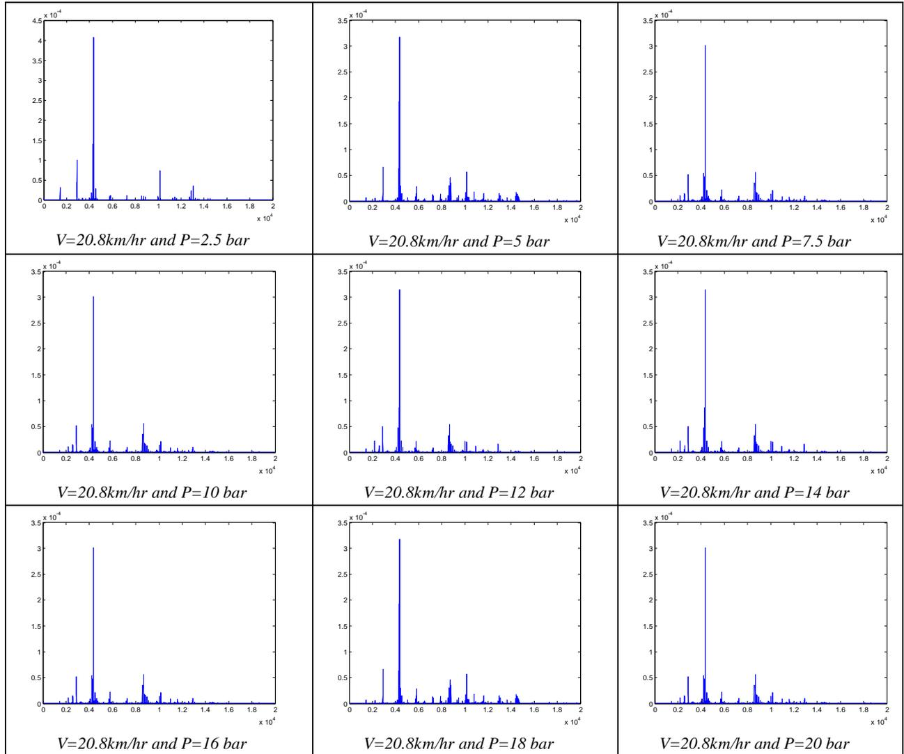
Fig.3(c) Effect of applied load on vibration at vehicle speed of 20.8km/hr.
