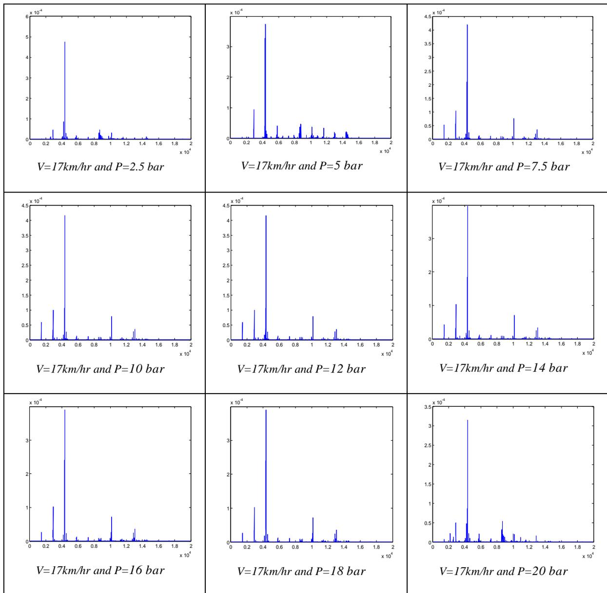
Fig. 3(b) Effect of applied load on vibration at vehicle speed of 17km/hr.
