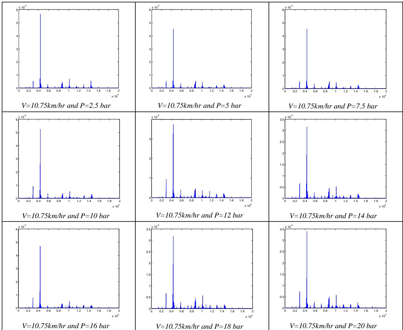
Fig. 3(a) Effect of applied load on vibration at vehicle speed of 10.75km/hr
